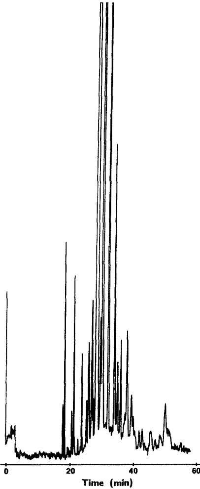
Fig. 7. Electrophoretic separation of enzymatically digested hyaluronic acid in a polyacrylamide gel-filled capillary. Gel concentration, 15% T, 3% C. Capillary, 39 cm (25 cm effective length) \times 50 \mu m I.D.; buffer as in Fig. 6; applied field, 282 V/cm (10 \mu A).
